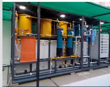
The Electrolytic Scale Remover (ElSr) by Venlar Corporation uses advanced electrolytic technology to control bio contamination, eliminate scale buildup, and improve energy efficiency in cooling tower water treatment without the use of harsh chemicals.
